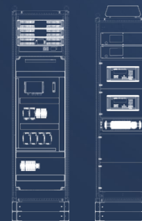
Cabinets for metering systems as a part of hydrocarbon, water, and steam metering units (information computation systems, information processing systems)
